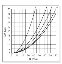
The diagram at the side shows the pressure drop curves for spools during normal usage. The fluid used is a mineral oil with a viscosity of 46 mm<sup>2</sup>/s at 40°C; the tests have been carried out at a fluid temperature of 40°C. For higher flow rates than those in the diagram, the losses will be those expressed by the following formula:
