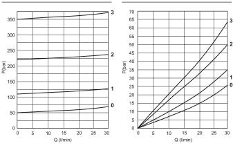
**0** = CMP04\*0 - **1** = CMP04\*1.. - **2** = CMP04\*2.. - **3** = CMP04\*3.. Fluid used: mineral based oil with viscosity 46 mm<sup>2</sup>/s at 40°C.
