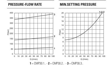
Fluid used: mineral based oil with viscosity 46 mm<sup>2</sup>/s at 40°C.
