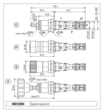
The valve has a combined function in a single cartridge. It consists of a direct acting maximum pressure valve and a unidirectional check valve.
