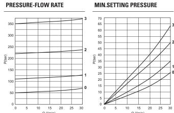
**0** = CPMC04\*0 - **1** = CPMC04\*1.. - **2** = CPMC04\*2.. - **3** = CPMC04\*3.. Fluid used: mineral based oil with viscosity 46 mm²/s at 40°C.
