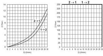
Fluid used: mineral based oil with viscosity 46 mm<sup>2</sup>/s at 40°C.
