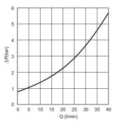
Fluid used: mineral based oil with viscosity 46 mm<sup>2</sup>/s at 40°C.
