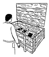
On receipt of the machine, check that it corresponds with order specifications, and that the packaging and contents have not been damaged during transport.
