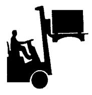
If the packed gear units are unloaded from a fork-lift truck, make sure the weight is balanced on the forks.
