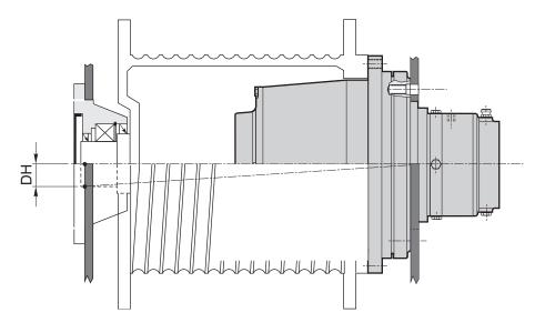
• The drum support bearing located on the opposite side of the gearbox must never be immobilised in an axial direction. The bearing must be free to slide axially to avoid unacceptable overloads acting on the winch or inside the gearbox.
