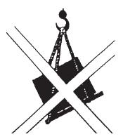
Do not tilt or turn the pack upside down while lifting or during transport.
