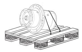
To move the packed gearbox, use lifting equipment that is suitable for the type of packing and having adequate lifting capacity, which must be indicated on the equipment, in relation to the weight of the load.
