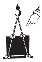
If the packs are unloaded with a hoist or, in any case, with a hook, make sure that the load is balanced and sling is using legally approved lifting accessories. For packs shipped on pallets, make sure that the lifting accessories do not damage the machine.
