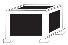
If necessary, place wooden chocks under the pack to facilitate lifting operations.
