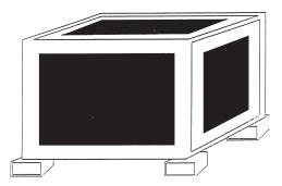
• If possible, insert wooden chocks between the pack and the floor.
