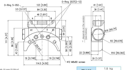
\*\* METRIC VERSION 3/8 G (BSPP) thread depth 15 mm [0.59 in] SAE VERSION 3/4-16 UNF thread depth 15 mm [0.59 in]
