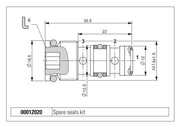
The shuttle type cartridge valves allow taking of the highest pressure signal to the external port via displacement of ball in tempered and ground steel. There are usually employed to signal the actuator load to a load sensing pump pressure compensator. External steel body protected on surface by zinc plating.
