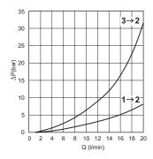
Fluid used: mineral based oil with viscosity  $46\ mm^2/s$  at  $40\ ^{\circ}C.$
