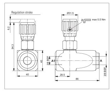
The valve maintains the flow rate in one direction (A to A1) regardless of oil pressure; the oil flows freely in the opposite direction.
