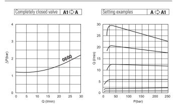
Fluid used: mineral based oil with viscosity 32 mm<sup>2</sup>/s at 40°C.
