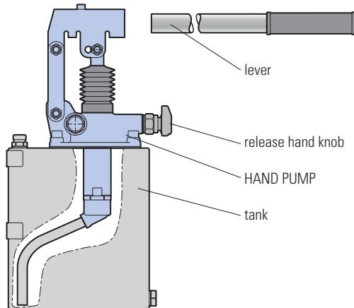
Hand pump for fixing to wall (without lever\*)
