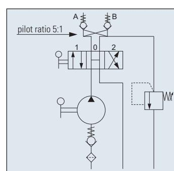
**HAND PUMP WITH 4/3 FLOW DIVIDER, DUAL PILOT CHECK VALVE, BRAKES
