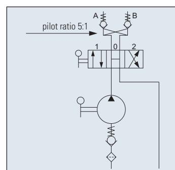
**HAND PUMP WITH 4/3 FLOW DIVIDER, DUAL PILOT CHECK VALVE, BRAKES
