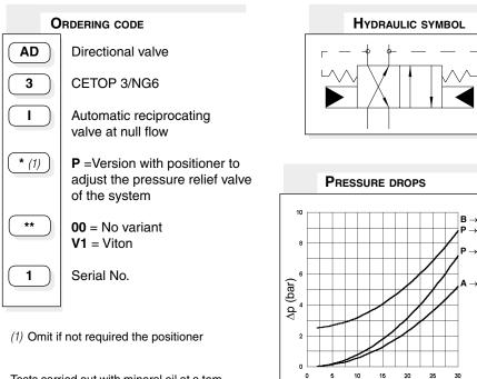
Tests carried out with mineral oil at a temperature of 40°C with viscosity of 46 mm<sup>2</sup>/s.
