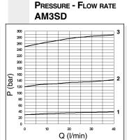
The fluid used is a mineral based oil with a viscosity of 46 mm²/sec at 40 degrees C. The tests have been carried out at with a fluid temperature of 40 degrees C.
