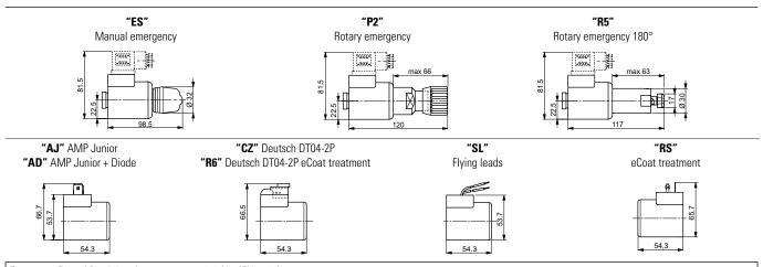
Emergency P2 and P5, tightening torque max.  $6 \ensuremath{\div} 9$  Nm (CH n. 22)
