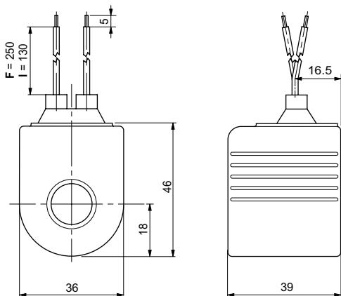
**WIRES and integrated bidirectional DIODE (F/I connection - FL/LD variant)**
