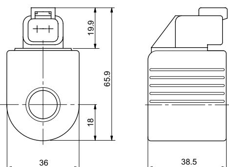
**DEUTSCH + bidirectional DIODE - DT04-2P (D connection - CX variant)**
