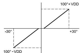
In order to obtain the output signal from the joystick as indicated in the diagram it is necessary: connect the Pin B of the connector at +VDD, and connect the Pin D at -VDD.
