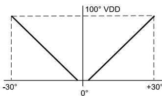
In order to obtain the output signal from the joystick as indicated in the diagram it is necessary: connect the Pin B and Pin D of the connector at +VDD, and connect the Pin A at 0V.
