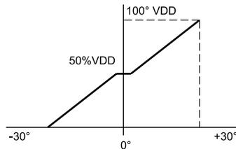
In order to obtain the output signal from the joystick as indicated in the diagram it is necessary: connect the Pin B of the connector at +VDD, and connect the Pin D at 0V.
