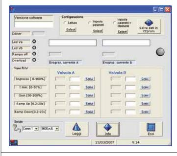
DG program for the digital adjustment of the parameters of the REMS and REMD boards.
