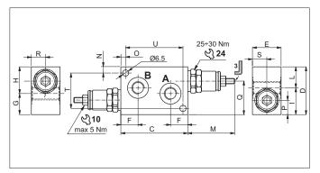
The direct acting compensator valves with CMP04 series 2 type cartridge protects the hydraulic components from impact or peaks in pressure.
