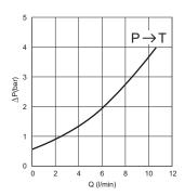
Fluid used: mineral based oil with viscosity 32 mm $^2$ /s at 40 $^{\circ}$ C.
