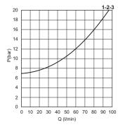
1 = VMP30.1.. - 2 = VMP30.2.. - 3 = VMP30.3.. Fluid used: mineral based oil with viscosity 46 mm<sup>2</sup>/s at 40°C.
