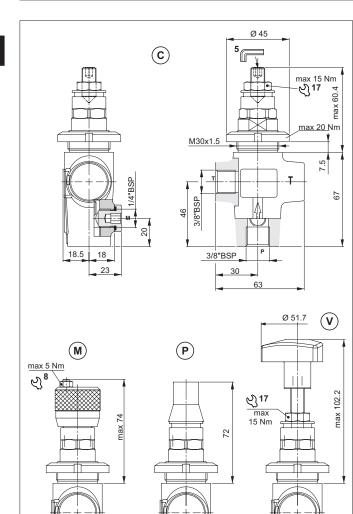
The direct acting relief valve with CP06 cartridge limits the pressure in the hydraulic circuit.
