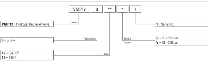
The pilot-operated relief valve limits the pressure in the hydraulic circuit. Slight leakage is tolerated for this type of valve.
